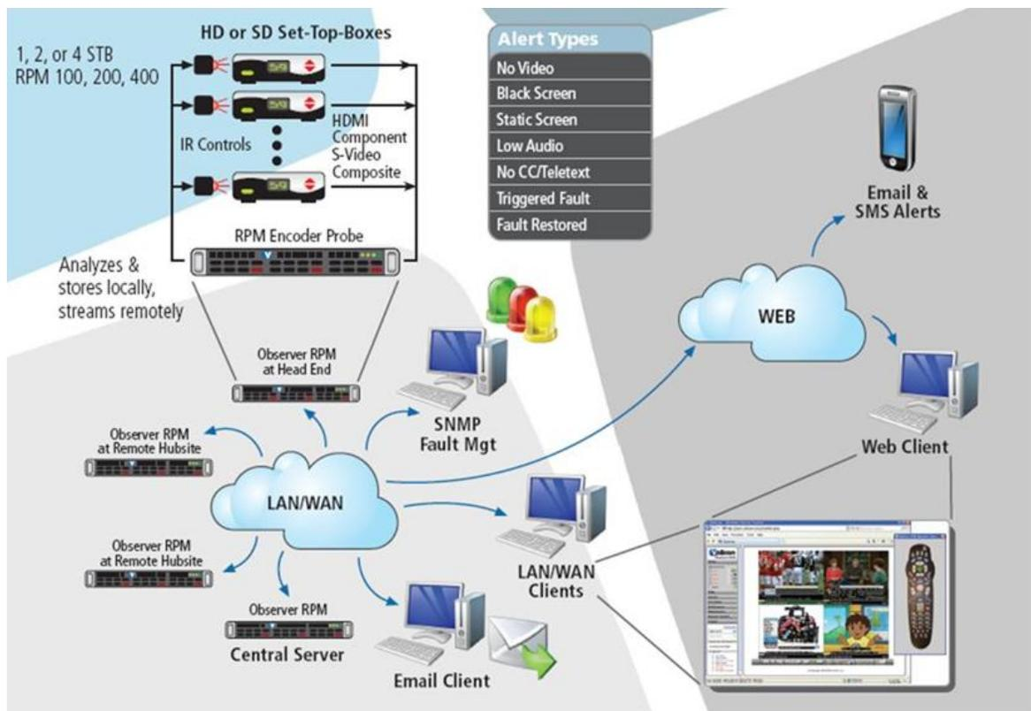
**Figure: RPM system components in a typical network**
