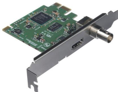
*Figure: Decklink Mini Monitor Output Card*
