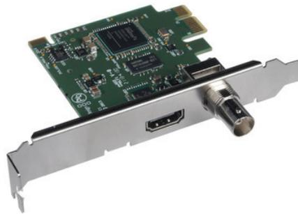
*Figure: Decklink Mini Recorder Card*
