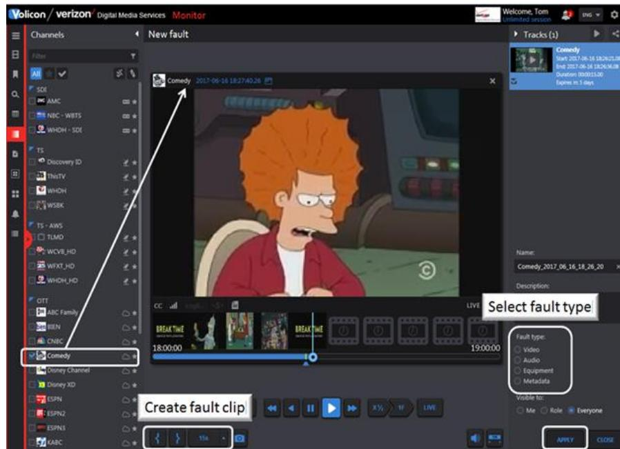
**Figure: Manual fault clip creation**
